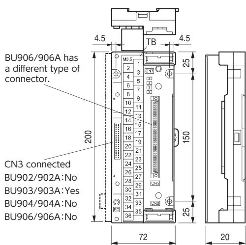
(Note 1) BU902A/903A/904A/906A can have a common bar/short bar attached, but be sure to allow sufficient space for the wiring terminal which may protrude up to 20mm on the left side.
